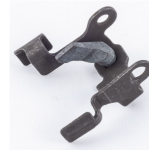
APX OVERSIZE HOLD OPEN #C7A136 ~2mm more protruding on both levers (right and left)
